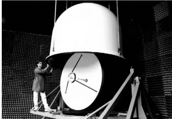
Fig. 1 Installation of radome over the antenna
