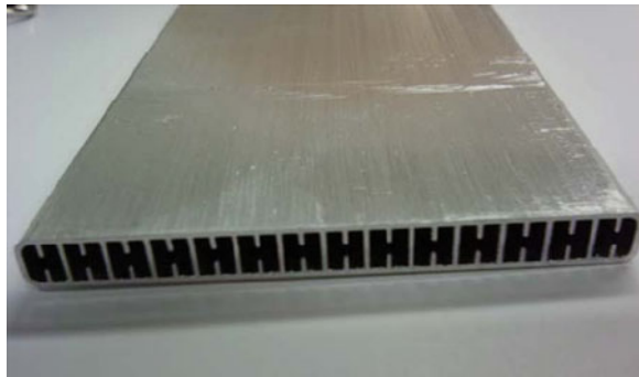
Fig. 7 Aluminum section of cold plate
