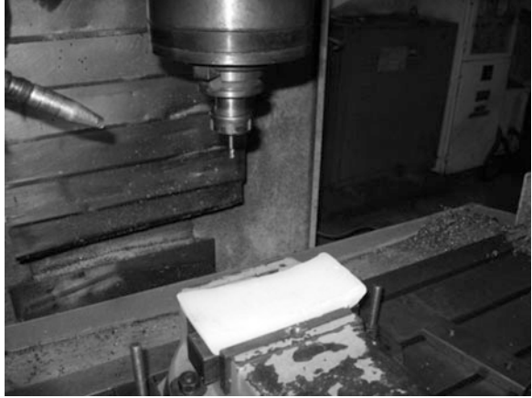
Fig. 9 Work piece and tool setup
