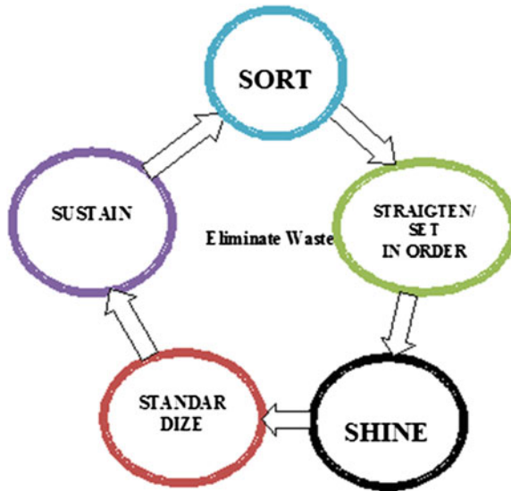
Fig. 2 Relation of 5S with waste elimination
