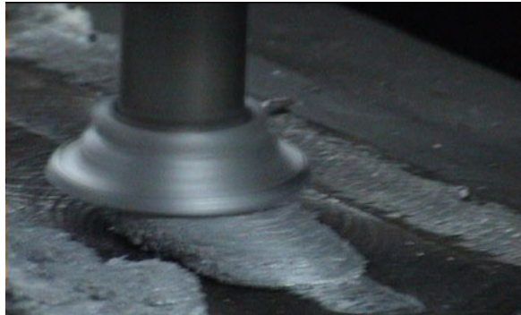
Fig. 3 Coating of aluminium over mild steel
