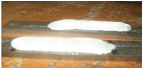
Fig. 4 The formation of layers along the plate after coating of aluminium over mild steel
