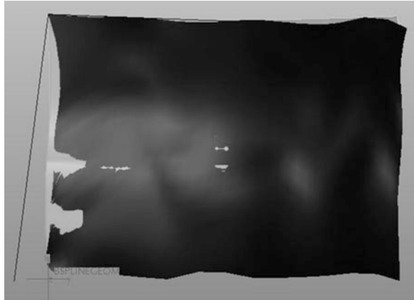
Fig. 12 Overlapping of B-spline machined and desired surface
